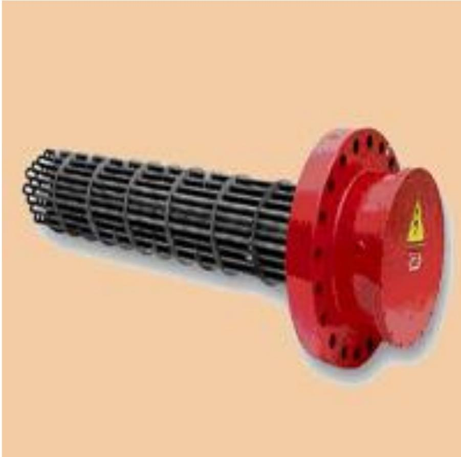
Ideal for generating steam and heating gases and liquids in pressure vessels and tanks, flanged immersion heaters are hairpin-bent tubular elements welded or brazed into a flange and provided with electrical enclosures. And Engineers flanged immersion heaters are available in a wide selection of flange sizes and with a variety of electrical enclosures.
