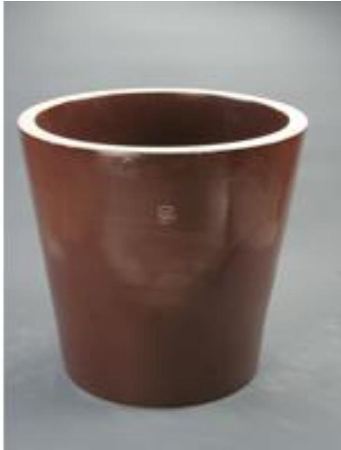
We provide conical support insulator for almost all type of ESP up to total height of 750mm. Suitable to withstand vertical load up to 08mt and 400°C temperature.
